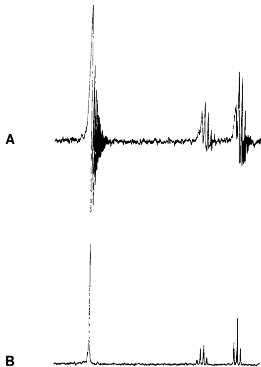
Fig. 1. Rapid scan spectrum of ethyl benzene before (A) and after (B) correlations.
